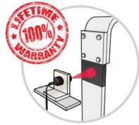
Infrared Sensors Monitor Busbar Joints
